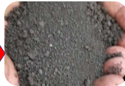
Output : ETP Sludge at 15~20% Moisture
