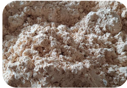
Input : WTP Sludge at 70% Moisture
