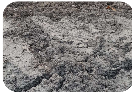
Input : ETP Sludge at 75% Moisture
