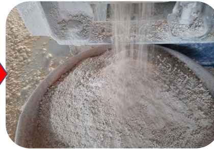
Output : WTP Sludge at 15% Moisture
